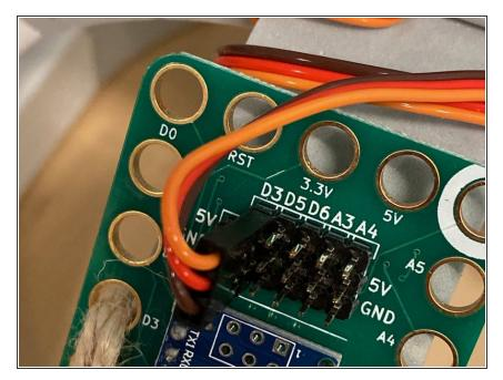
Connect the motor to D3 as shown.
